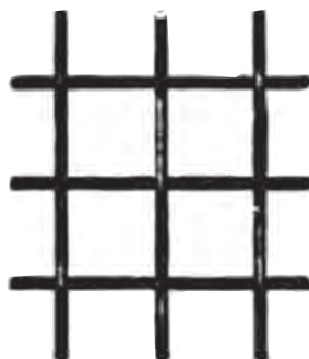
2 mesh opening .4375 in. .0625 in. dia. wire
