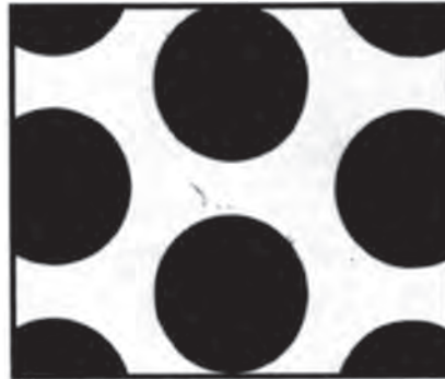
\frac{3}{4} " diameter. 1" staggered centers. 1.1 holes per sq. inch. 51% open area.
