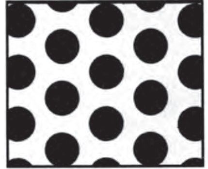
3/8" diameter. 5/8" staggered centers. 4 holes per sq. inch. 40% open area.
