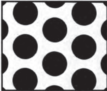
1/2" diameter. 1/4" staggered centers. 2.5 holes per sq. inch. 48% open area.
