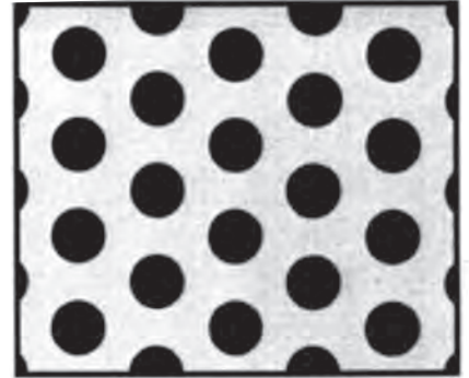
1/4" diameter. 7/16" staggered centers. 6.5 holes per sq. inch. 32% open area.
