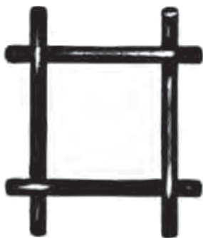
1 in. mesh opening .8650 in. .1350 in. dia. wire
