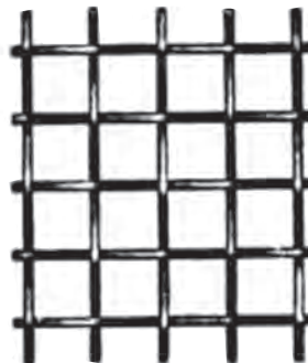
3 mesh opening .2793 in. .0540 in. dia. wire
